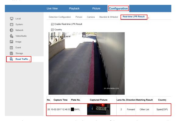
In this instant-view you can see the date and time of the capture, the Registration Plate as read by the OCR, the captured image of the same, the lane number in which the detection
