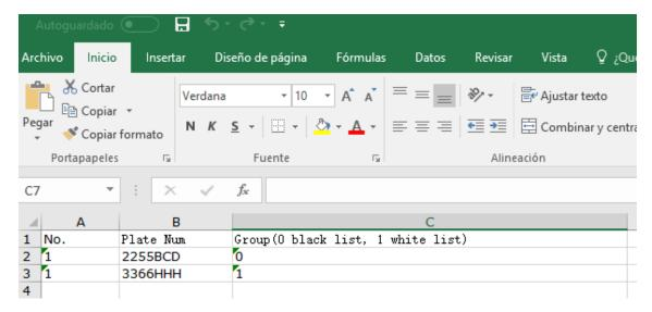
When your Excel table is completed you can import it into the system (in the same location, "Configuration" / "Road Traffic") by selecting "Browse". You will be prompted to select the Excel spreadsheet with the Number Plate database. Then click on "Import" to complete the vehicle List configuration.
