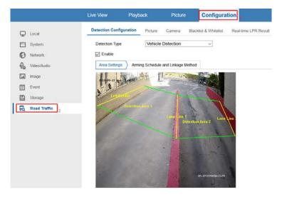
Activate the Number Plate detection by clicking on the "Enable" check-box, as shown in the following screenshot:
