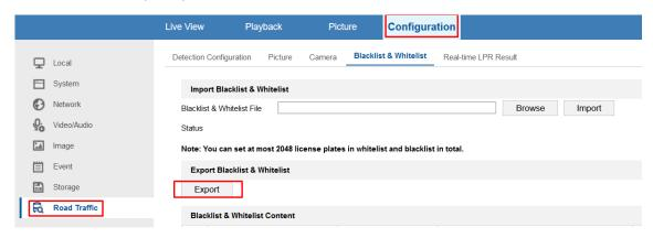
In the Excel sheet, spaces and hyphens should NOT be used. To assign a Number Plate to the White List, place a 1 in the "group" column, however, if you want to put the Number Plate in the Black List, then a 0 (zero) will be entered in the column (See sample image below).
